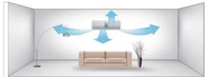
The louver can be vertically or horizontally adjusted so as to maximize comfort in the room.
